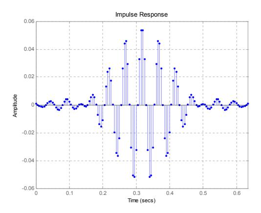
Figure LM6-6 Impulse response of an FIR filter
