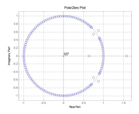
Figure LM6-3 Pole-zero map of an FIR filter with 127 taps
