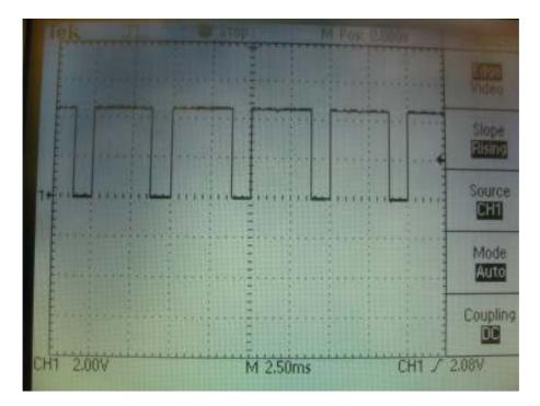
Figure LM6-13 Measuring the execution time of the filter algorithm
