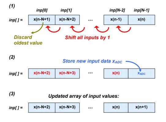
Figure LM6-10 Updating the input array inp[]
