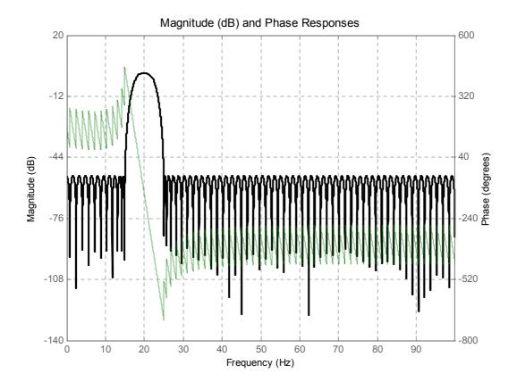
Figure LM6-4 FIR filter response, magnitude (bold) and phase (fine)
