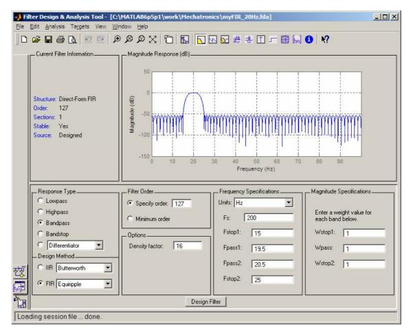
Figure LM6-2 Using MATLAB to determine the filter coefficients (fdatool)
