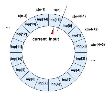
Figure LM6-11 Ring buffer structure for a 16-elements filter array
