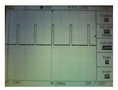
Figure LM6-15 Evaluating the execution time of the IIR filter
