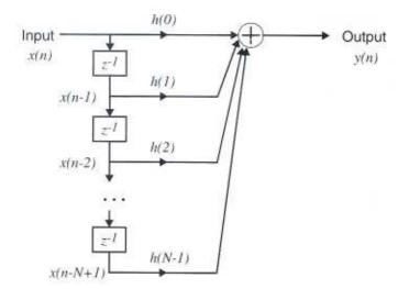
Figure LM6-8 FIR filter structure (direct form)
