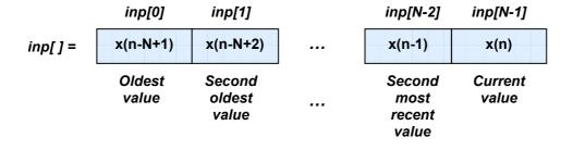
Figure LM6-9 Storing previous input values in an array variable
