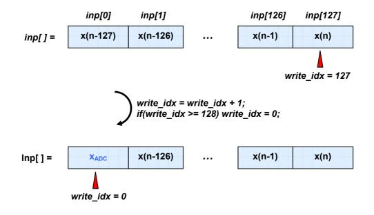
Figure LM6-12 Wrapping around at the end of the buffer
