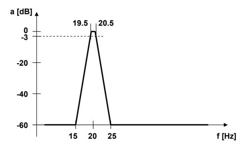
Figure LM6-1 Band-pass filter specification
