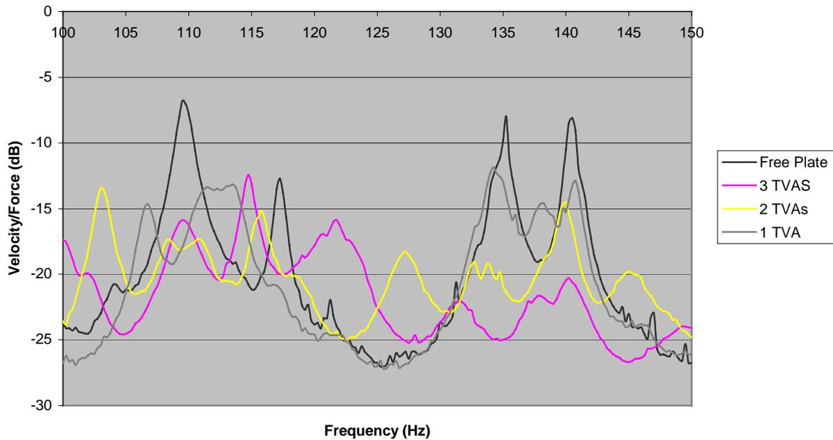
**Figure 5 Average Spectrum (Vel./Force) of plate using 4 different configurations**
