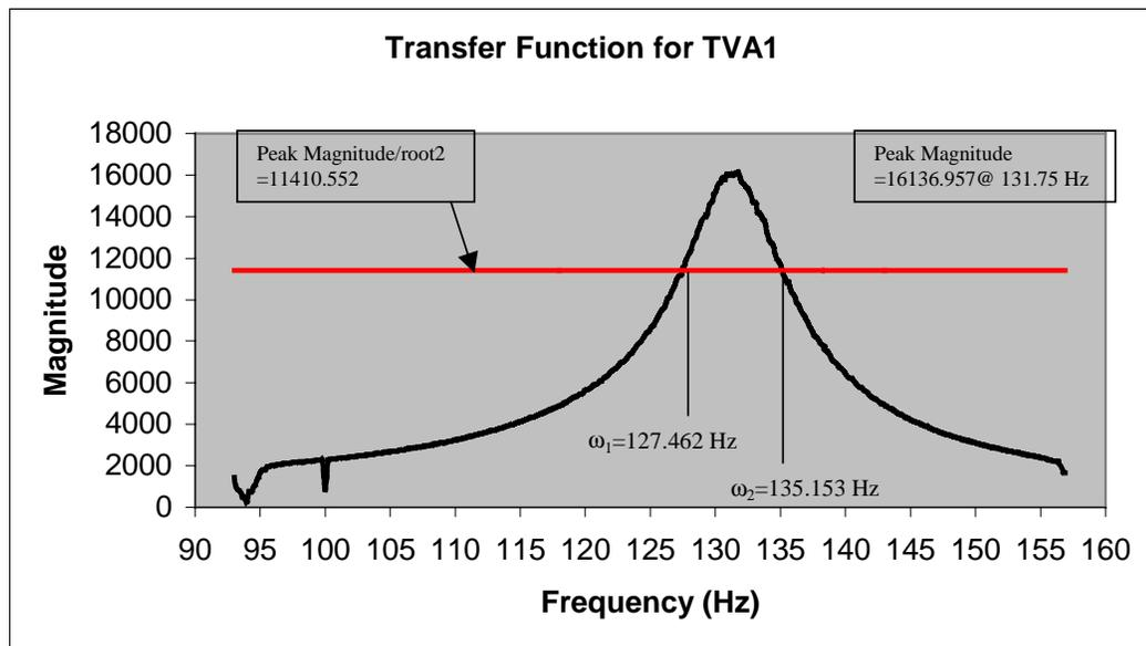
**Figure 3 Transfer Function X/Y for TVA1**
