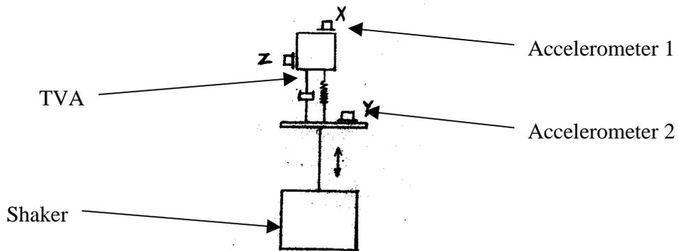
**Figure 2 Shaker Test Schematic Diagram**
