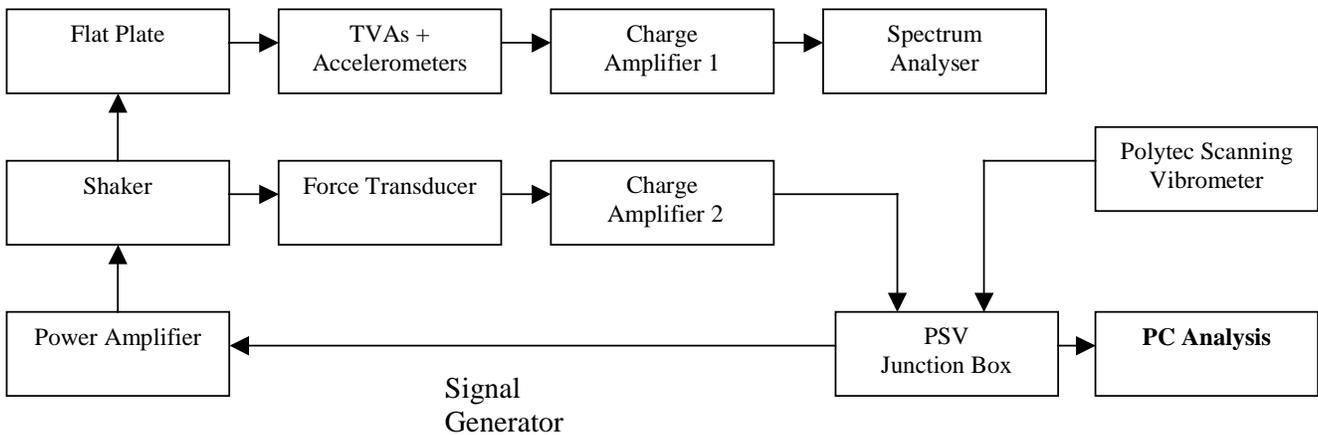
**Figure 4 Flat Plate Experiment Flow Diagram**
