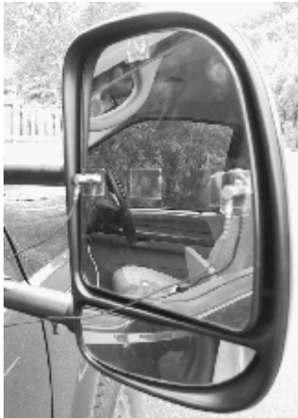
Figure 3 P131 mirror with accelerometers attached
