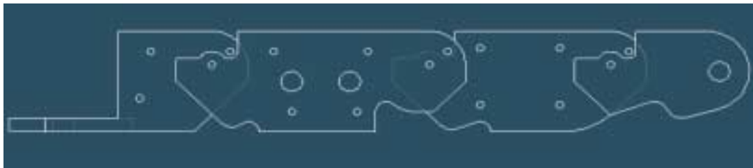
Figure 2: Finger Design Showing Mechanical Stops to Restrict Motion
